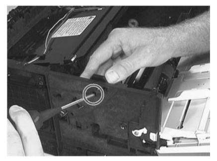
3 Slide the guide up and out to remove it (see figure 7-109).
