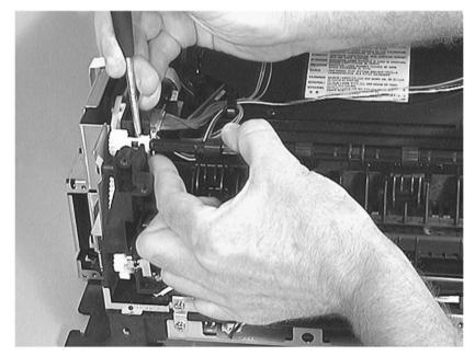
**3** Release both clips on the non-geared end of the roller's shaft while lifting it (see figure 7-58).
