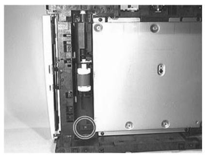
Figure 7-93 Removing Tray 2 Pickup Roller Assembly
