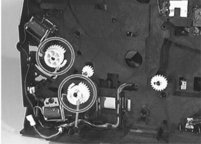
**3** Remove the black bushing shown in figure 7-80. While facing it, pull out its lever and rotate it clockwise until the tab clears the keyed opening.
