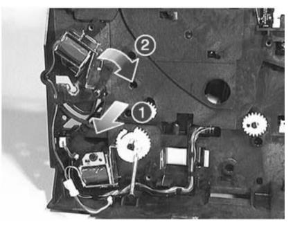
Figure 7-80 Removing Tray 1 Pickup Roller Assembly Black Bushing
