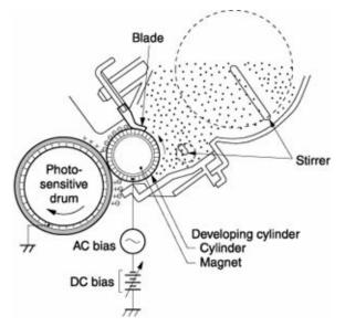
At the developing stage, the latent electrostatic image is developed into a visible image on the photosensitive drum. The developing cylinder consists of a metallic cylinder that rotates around a fixed magnetic core inside the toner cavity. Toner is a powdery substance made of black, plastic resin bound to iron particles, which the magnetic core of the developing cylinder attracts. A rubber blade brushes the toner on the developing cylinder to a uniform thickness.
