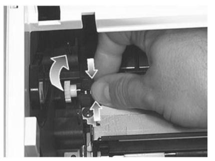
Figure 7-5 Removing the Transfer Roller (1 of 2)
