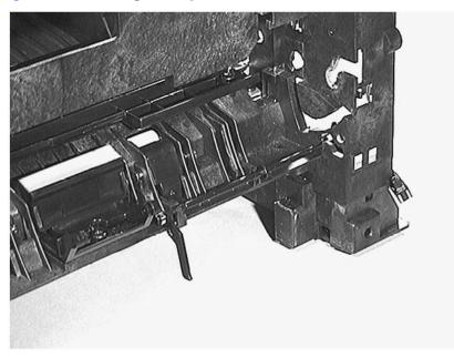
Figure 7-89 Setting the Paper Sensor Lever in its Cradle
