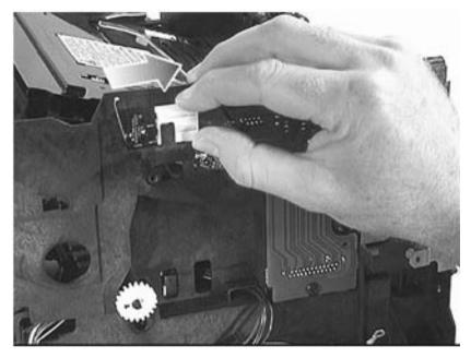
**3** Disconnect the power cables from the laser scanner and the cooling fan at the location shown in figure 7-96.
