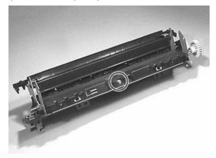
4 Lift and remove the pressure roller.
