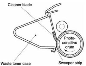
At the cleaning stage, the photosensitive drum's surface is prepared to hold an image. During printing, the drum rotates completely several times per printed page. Before forming the image for a given section of print, a cleaning blade removes toner from the previous rotation of the drum. The toner cartridge stores waste toner and prevents it from being used in later print jobs (see figure 5-9).
