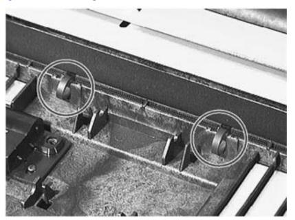
Figure 7-67 Installing the A-1 Belt and Roller
