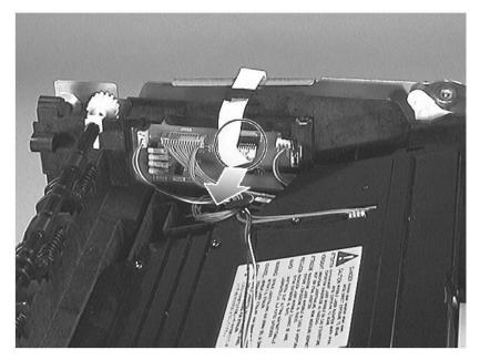
**3** Lift the tab shown in figure 7-72, and then slide the ribbon cable harness to the right to remove it.
