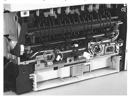
Figure 7-38 Removing the Fusing Assembly's Screws
