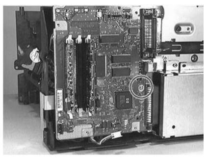
Figure 7-28 Removing the Formatter PCB
