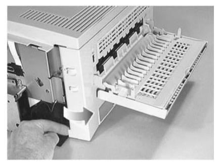
5 Pull the rear cover down and then out to remove it.
