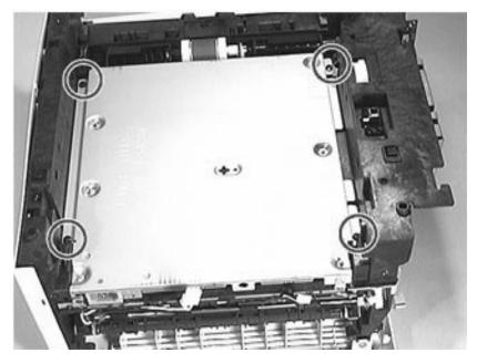
7 Lift the left side of the engine controller assembly. All of the wire connectors are attached to the right side of the engine controller assembly.
