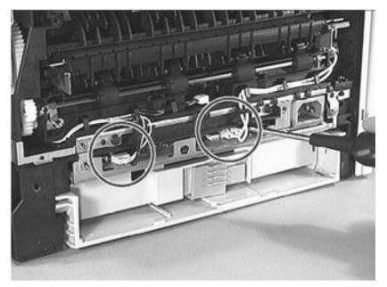
4 Remove the two grounding plate screws shown in figure 7-48.
