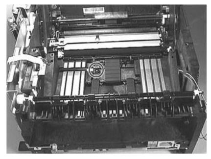
**3** Lift the center shaft (see figure 7-64) out of its carriage and gear box.
