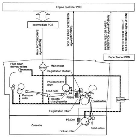
PS502: Top of page sensor (Printer PS2001: Paper feeder paper sensor
