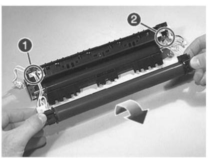
Figure 7-44 Removing the Fusing Film
