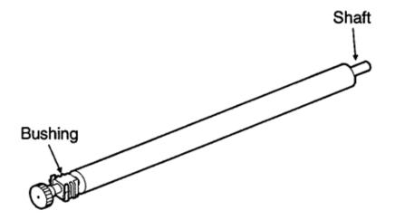
4 Squeeze both of the black bushing's tabs (see figure 7-5), and then lift the transfer roller's shaft to the left (see figure 7-6).
