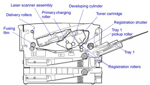
Figure 1-7 Internal Assembly Locations (2 of 2)
