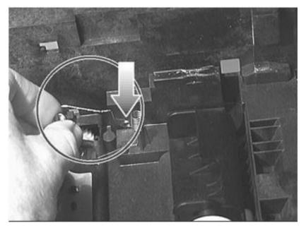
Figure 7-126 Inserting the Spring through the Opening (2 of 2)
