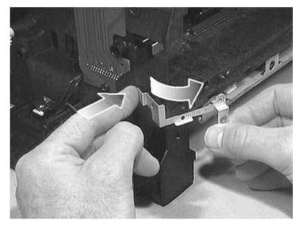
Figure 7-102 Fusing Assembly Ground Clip
