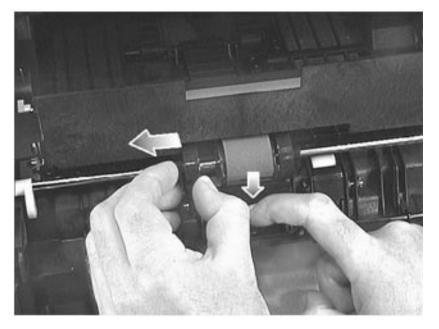
6 Press and hold the release mechanism (see figure 7-117) on the pickup roller, and then slide it to the right (see figure 7-118).
