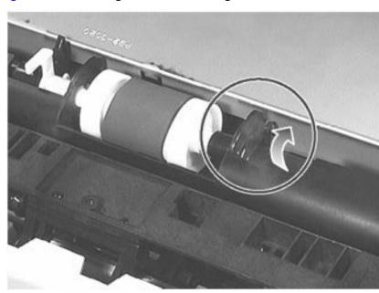
Figure 7-21 Locking the Black Bushing in Place
