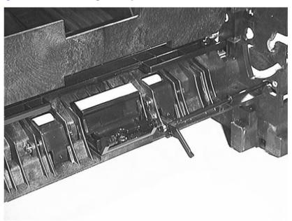
Figure 7-87 Removing the Paper Sensor Lever
