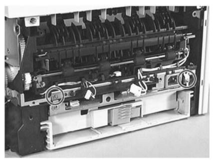
Figure 7-37 Removing the Fusing Assembly's Grounding Plate Screws
