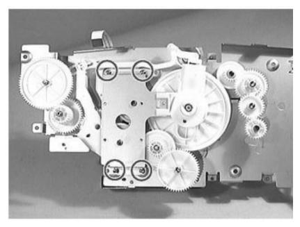
**3** Press and hold the clip shown in figure 7-77, and then slide the motor plate out of the plastic holder while holding the bushing down with the other hand.
