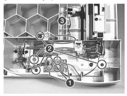
Figure 7-132 Removing Tray 3 Wire Connectors and Screws
