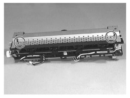
**5** Press the clips shown in figure 7-43 to remove the pressure plate.
