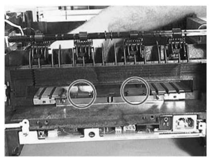
Figure 7-68 Installing the B-1 Belt and Roller
