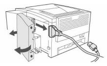
**3** Locate the EIO Slot. Firmly insert the HP JetDirect EIO card into the EIO slot. Twist in the retaining screws.
