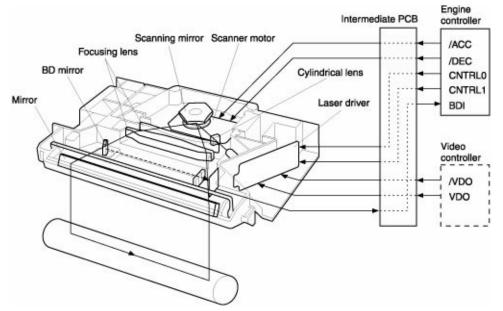
At the Laser Scanner, a laser beam focuses onto the photosensitive drum and discharges the drum's negative potential. This creates a latent electrostatic image, which later is developed into a visible image.
