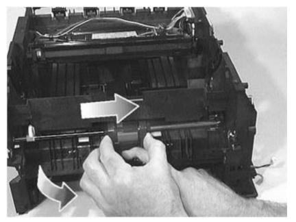
Figure 7-82 Removing Tray 1 Pickup Roller Assembly
