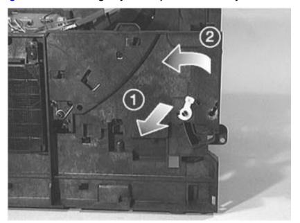
Figure 7-81 Removing Tray 1 Pickup Roller Assembly White Bushing
