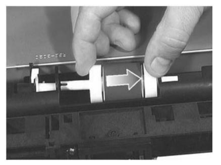
**10** To remove the pickup roller from its carriage grasp the left end of its shaft and then lift up the roller.
