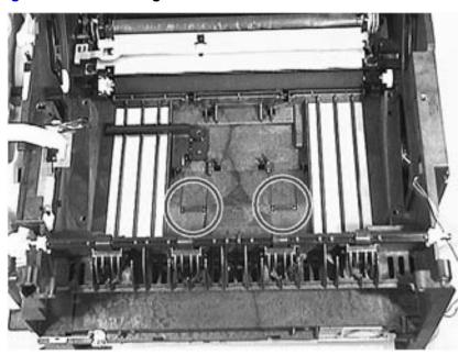
Figure 7-65 Removing Small Rollers
