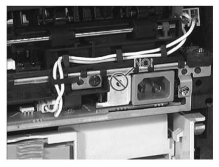
Figure 7-34 Not a Print Engine Test Button
