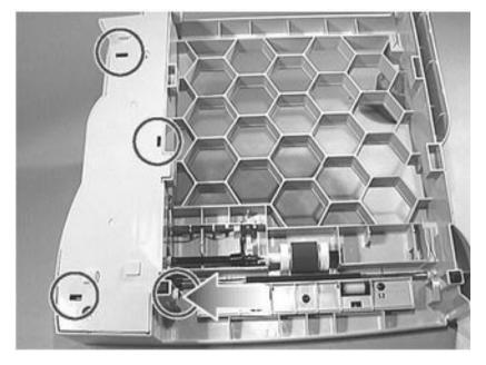
**3** Disconnect the three wire connectors shown in figure 7-132.
