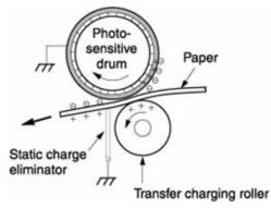
At the transferring stage, the toner image on the photosensitive drum's surface is moved to the paper. The transfer roller applies a positive charge to the back of the paper, causing the paper to attract the negatively charged toner on the drum's surface.
