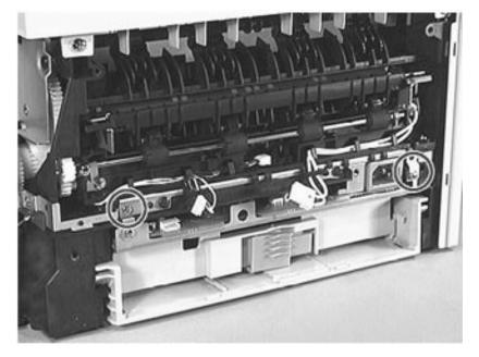
Figure 7-48 Removing the Fusing Assembly's Grounding Plate Screws
