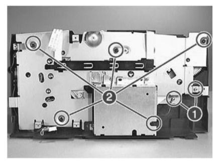
Figure 7-74 Removing the Printer Drive Assembly's Screws
