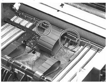
Figure 7-69 Installing the Non-Geared Roller Shaft
