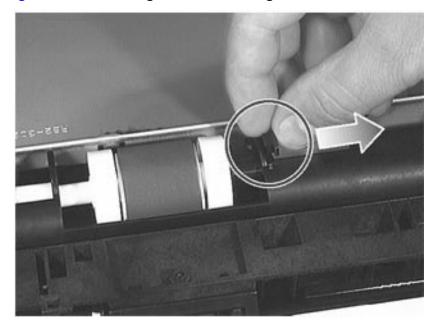
9 Slide the pickup roller to the right so that its shaft is removed from the white bushing.
