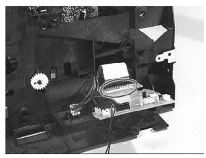
Figure 7-98 Disconnecting the Intermediate PCB's Ribbon Cable
