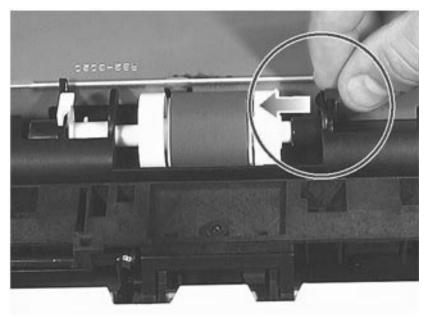
6 Rotate the black bushing forward until it locks in place.
