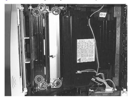
Figure 7-100 Removing the Registration Assembly's Screws
