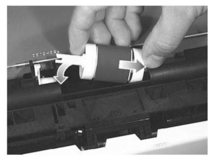
4 Slide the slotted end of the pickup roller's shaft into the white bushing. Rotate the roller while sliding it so that its slotted shaft rests over the drive shaft.
