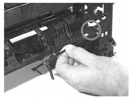
2 Set the paper sensor lever in its cradle as shown in figure 7-89. Make sure the spring is resting on the bottom of the printer.
