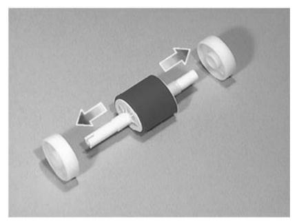
2 Place the two rollers on the ends of the new pickup roller.
