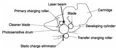
The toner cartridge contains the cleaning, conditioning, and developing stages of the image formation process. These components are subject to wear and are built into the replaceable toner cartridge. This eliminates the need for a service call when replacement is required.
