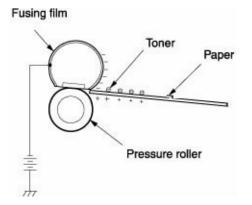
At the fusing stage, heat and pressure fuse the toner to the paper to produce a permanent image. The paper passes between a fusing film and a pressure roller. The fusing film melts the toner while the pressure roller compresses it into the paper.
