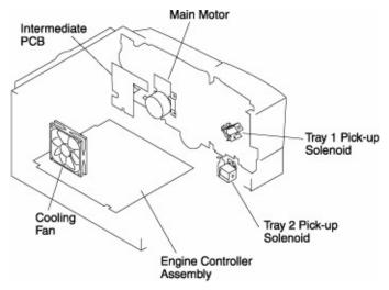
Table 6-11. Motor, Fan, PCB, and Solenoid Locations
