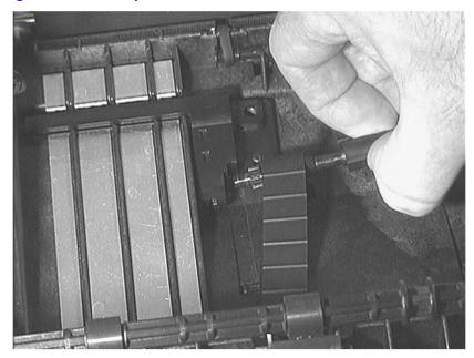
4 Remove all of the belts and rollers in any order. Do not overlook the two rollers located in the bottom of the printer (see figure 7-65). Lift each to remove it.
