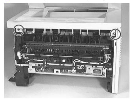
Figure 7-53 Removing Screws from the Top Cover (2 of 2)
