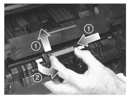
**3** Simultaneously squeeze both brackets to remove the separation pad from the swing arms.
