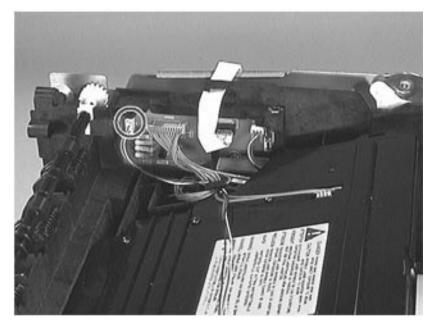
**3** Remove the two screws shown in figure 7-106.
