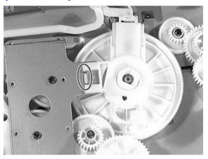
Figure 7-77 Removing the Motor Plate
