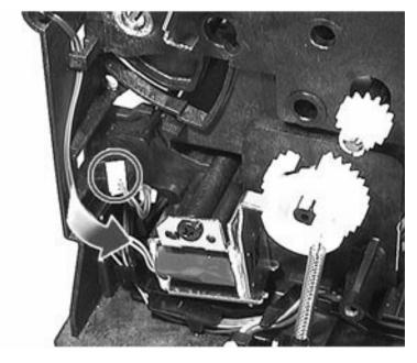
4 Pull the center of the paper sensor lever outward (see figure 7-86), and then slide it to the right until it stops.
