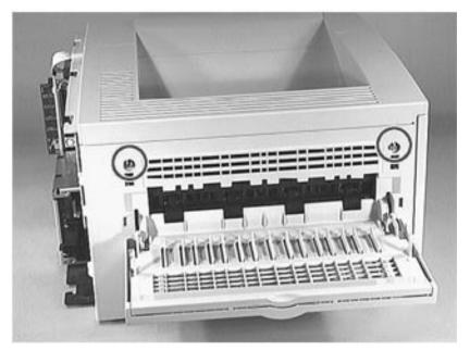
4 Pull the bottom-left corner of the rear cover as shown in figure 7-32.
