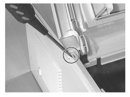
Figure 7-55 Releasing the Latch on the Top Cover
